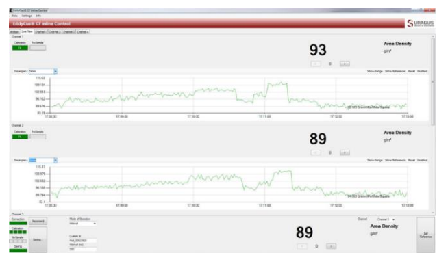
Basis weight monitoring of four lanes: two lanes diagrammed
